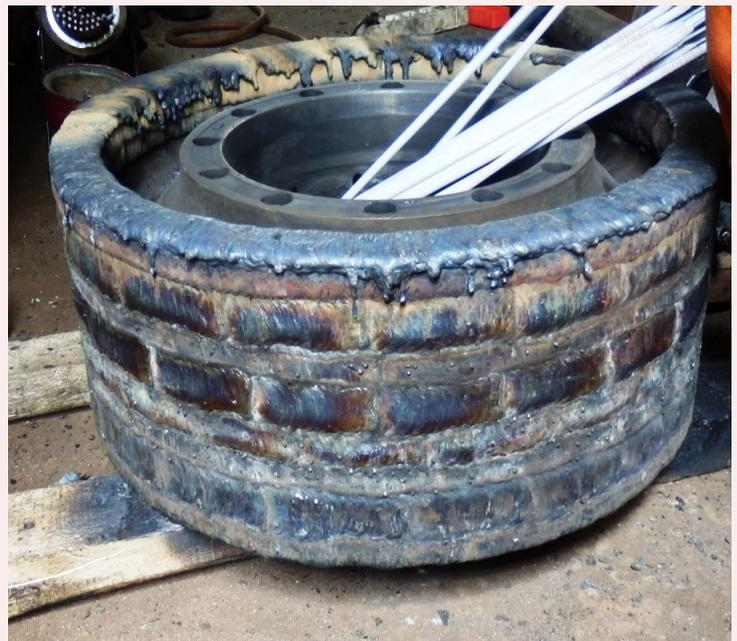
**Worn Piston crown totally rebuilt using ARCWEL E -808 stick electrode**
