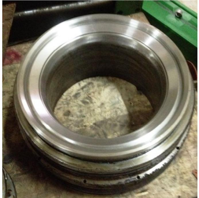
Valve coated using PTA Process
