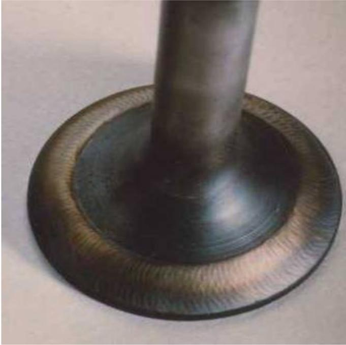
Valve seats rebuilt by GTAW Process,
